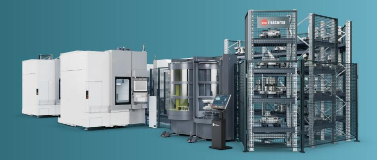
Flexible Pallet System is a modular CNC automation solution that enables lights-out manufacturing and high spindle utilization with 4- and 5-axis milling and mill-turn machine tools. What sets it apart from other solutions are its modular 360-degree design, integration capability with over 90 machine brands, and state-of-art MMS production planning capabilities. FPS can be extended or upgraded if there is a change in production needs.
