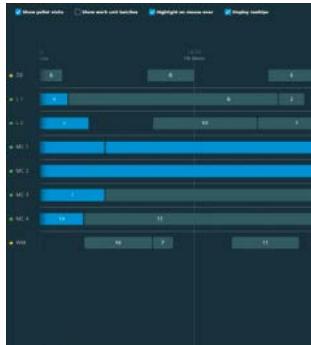
Intelligent production control software schedules the production based on ERP order due dates, and adapts to any changes in real time.
