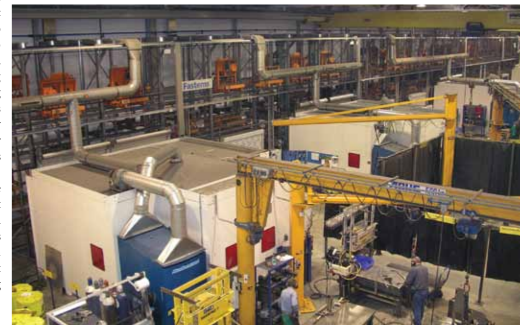
MLS-XMD: 67 m long, 6.3 m high, 152 welding pallets, 4 ABB welding robots, 8 binding and infeed/retrieval stations, ergonomic, simple, and safe.
