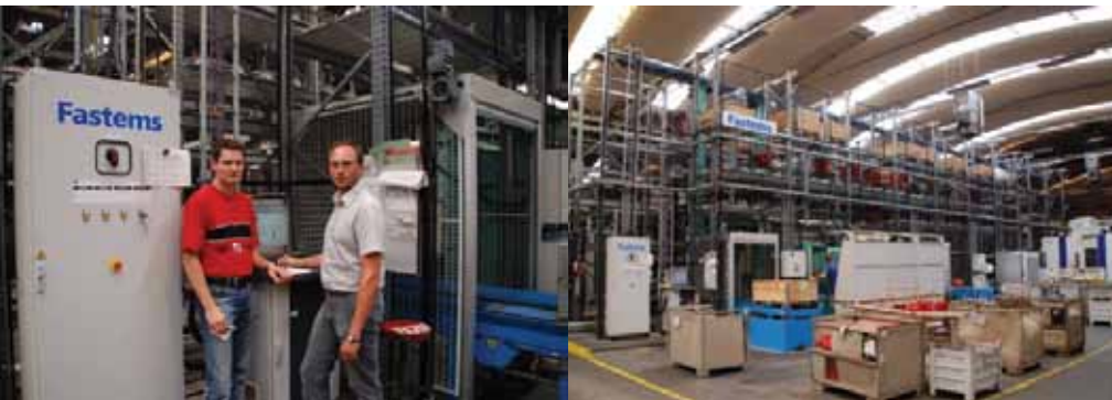
Left picture: Mr. Franz Eichinger - Leader of manufacturing engineering and fixture construction (right) and Mr. Oliver Steininger - Leader of mechanical production division I (left). Right picture: At present, the Fastems system has more than 117 pallet places, of which 89 are used for workpieces and 28 for raw material
