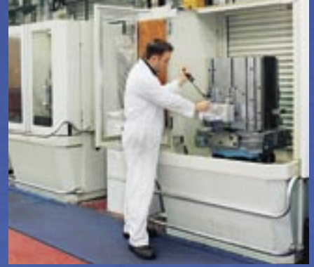
It is easy to clamp parts at a Fastems LSF loading station with a revolving pallet table.
